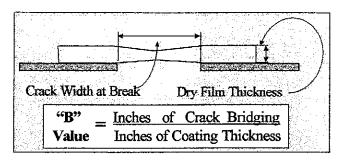
environment like Florida. The diagram to the right is an attempt to explain the concept, some chemist call it "B" value in the elastomerics field. In contrast to paints, our Aquathon, sporting its exceptional low temperature flexibility (down to -40°F) can bridge even a 1/8th wide crack in Minnesota when applied to a DFT of about 25 mils. In warmer markets 10-16 mils DFT can do the trick. Since Aquathon has high solids (50%)
